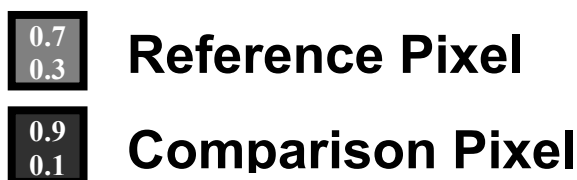
Figure 1 The reference pixel and comparison pixel with partial membership to the black category as specified by the top number and to the white category as specified by the bottom number within the pixel.
