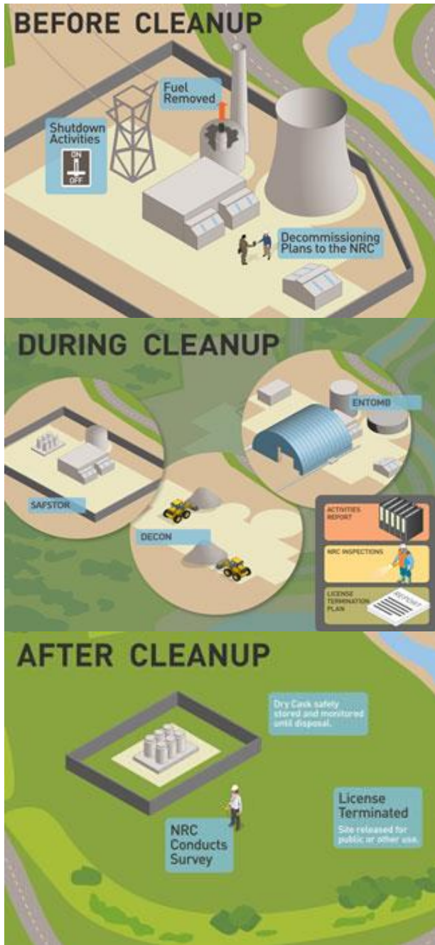
Figure 3. Basic outline of NRC decommissioning processes before, during, and after cleanup. (Retrieved from https://www.nrc.gov/reading-rm/doc-collections/fact-sheets/decommissioning.html#_ftnref1 )
