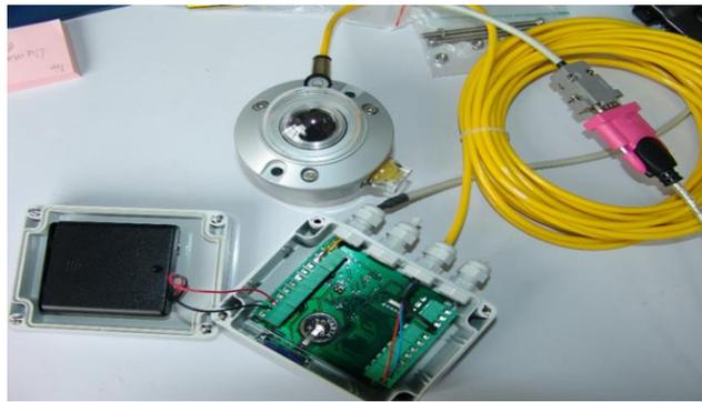
Figure 4 The connection of CMP-6
