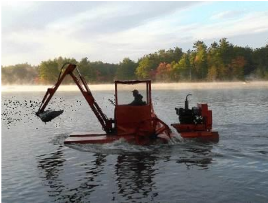
Figure 1. Hydro-raking machinery with seated driver (Foster's Pond Corporation, 2007).
