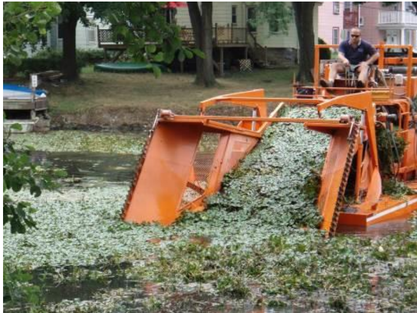
Figure 2. Harvester gathering plants onto conveyor belt. Photo credit: (Mystic River Watershed Association, 2010)
