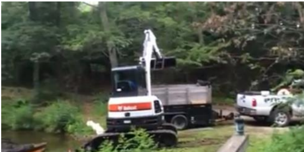
Figure 28. Video still showing plant debris removed from the barge by a loader bucket, deposited into a hauler, pulled by a truck. Video still credit: (Tom Largy, 2015a)
