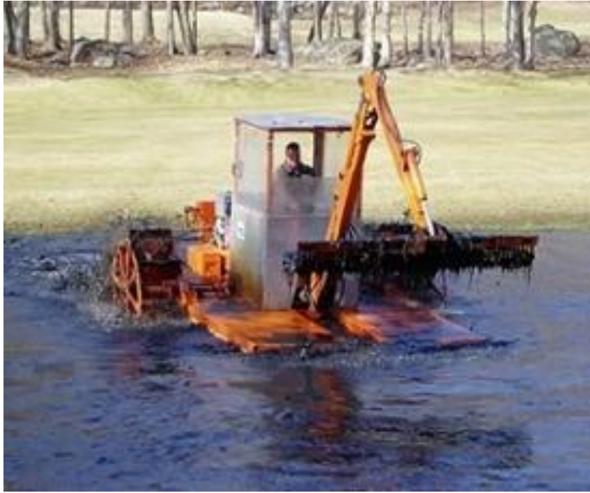
Figure 5. Hydro-rake removing plant debris from the water, showing the plastic water-guard up around the operator. Photo credit: (Solitude Lake Management, 2014a).
