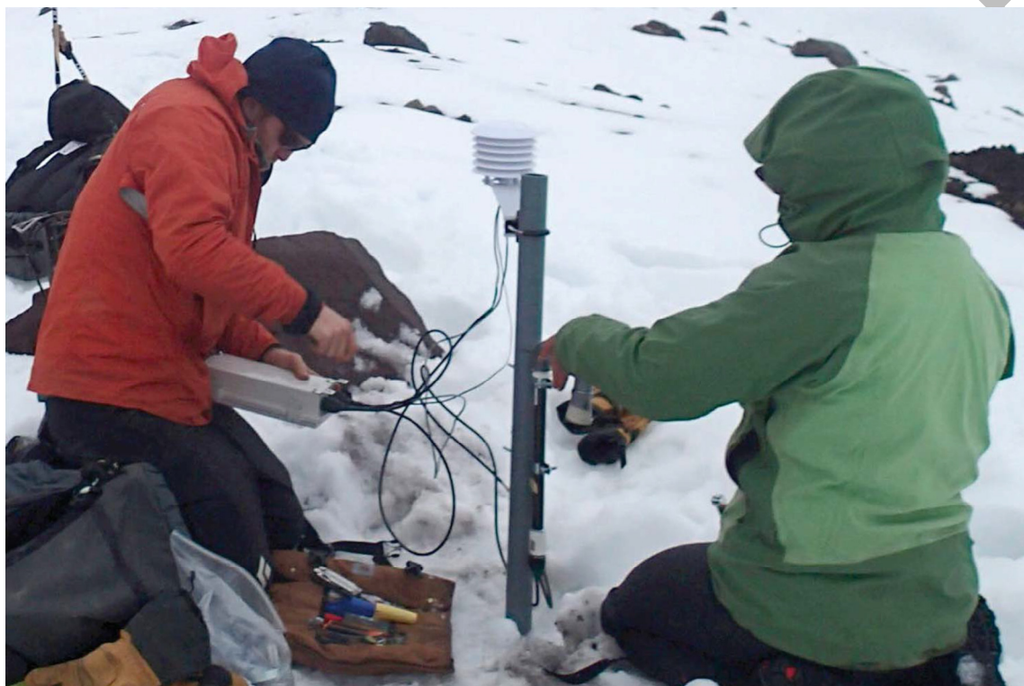
Figure 6. Andy Wickert (Left) and Rachel McLaughlin (Right) construct a glacier monitoring station to measure snow depth, ice melt, temperature, and relative humidity on Volcán Chimborazo, Ecuador, where tropical glaciers are rapidly retreating (La Frenierre and Mark 2017). The monitoring station is built from off-the-shelf components, and is centred around an open-source ALog data logger (inside the white box in AW's hand) that records measurements at constant time intervals. Expanding low-cost, low-power and off-the-shelf environmental monitoring tools is critical for data collection in remote areas (Wickert 2014), especially those that are experiencing rapid environmental change that threatens communities with limited resources (La Frenierre and Mark 2014).
