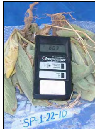
Fig. 11. SSGR checking a sample of leaves. --The Inspector should be bagged to protect it from contamination. [SSGR]
