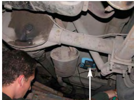
B. Inspector mounted under car
