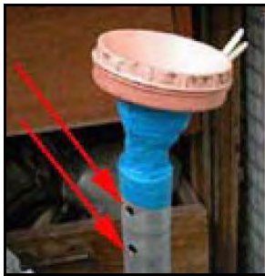
Fig. 9. On the left, a Russian air filter on a funnel, hooked to a Russian car vac on the right. See the Equipment list for possible U.S. equals. [SSGR]
