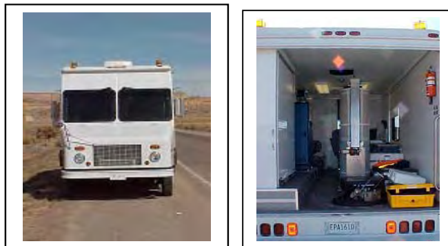
Figure III.3. Front and interior views of the USEPA gamma radiation Scanner Van used in the CRUMP radiation assessment.
